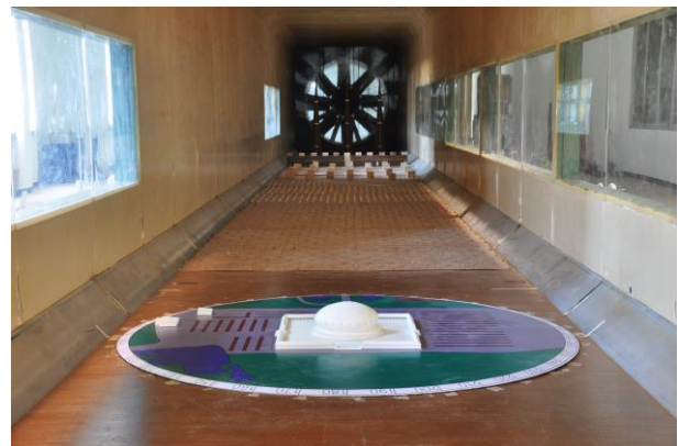
Figure 7. The scaled model in TU-AIT Boundary-Layer wind tunnel
